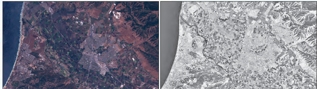
These Landsat-5 images depict the region surrounding Salinas, California in true color [left] and thermal infrared [right]. In the true color image, different types of agricultural fields (shades of green) surround the town of Salinas (shades of gray and white). In the thermal infrared image, warmer temperatures appear in bright shades (e.g., the town of Salinas), and cooler temperatures appear darker (e.g., some agricultural fields and the ocean).
